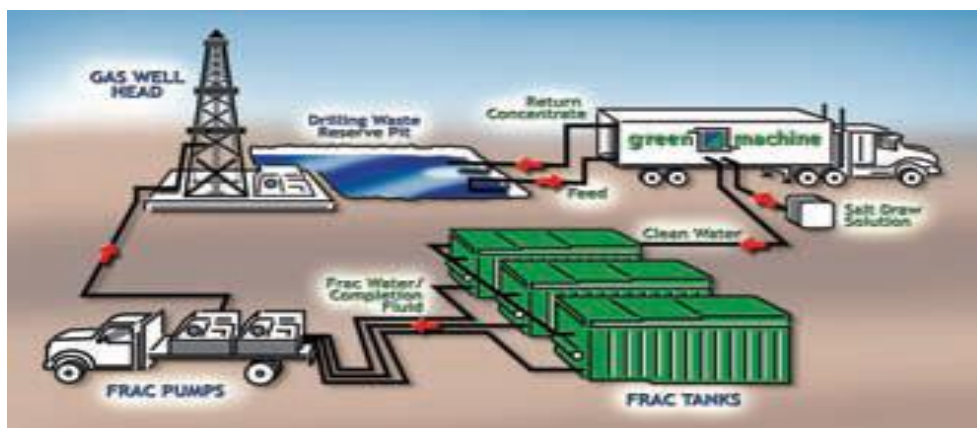
FIGURE 2 ILLUSTRATION OF FORWARD OSMOSIS SYSTEM, HOUSED AND TRANSPORTED IN LARGE TRUCKS LIKE THE ONE SHOWN ABOVE. IMAGE FOUND IN SOURCE [17].
