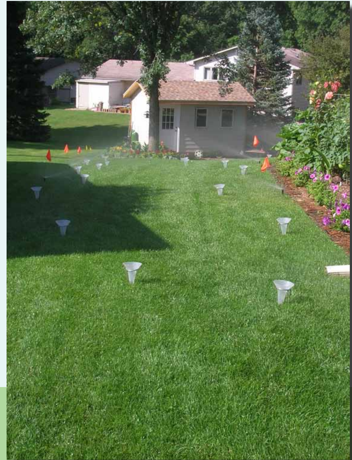
Irrigation uniformity measurement for residential irrigation sprinklers. Courtesy of Todd Trooien, Professor, South Dakota State University
