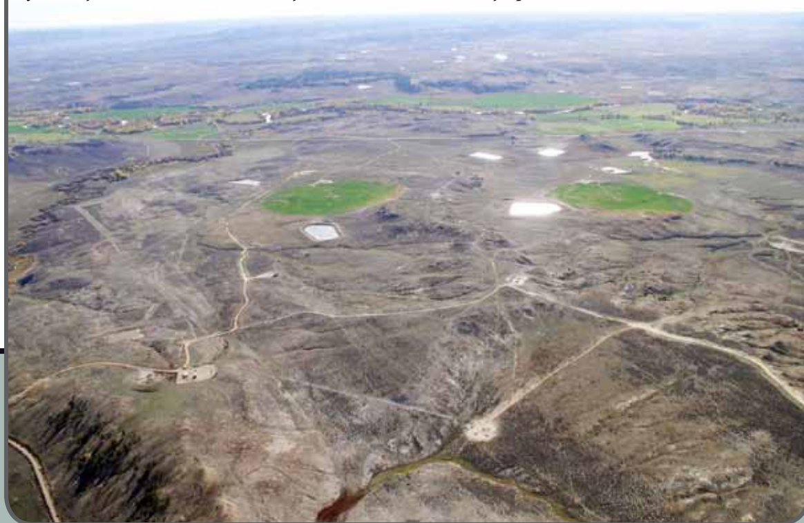
Constructed surface storage ponds and impoundments for coalbed methane product water along the Tongue River corridor, south central Montana. Courtesy of Jim Bauder, formerly Montana State University Extension Water Quality Specialist
